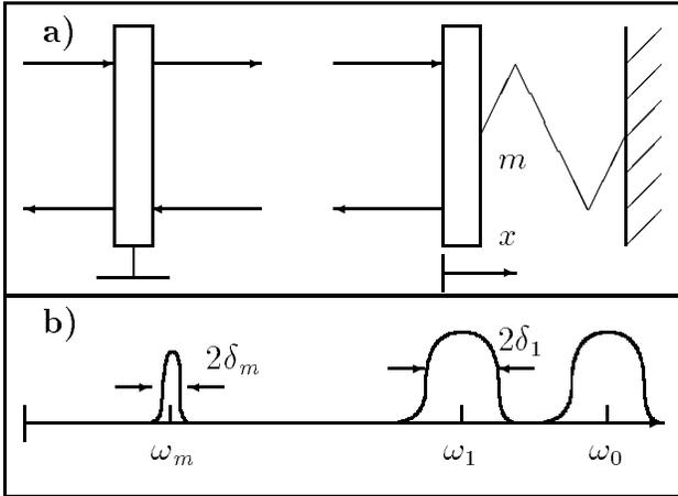
FIG. 10. Scheme of FP resonator with movable mirror (a) and frequency diagram (b).
