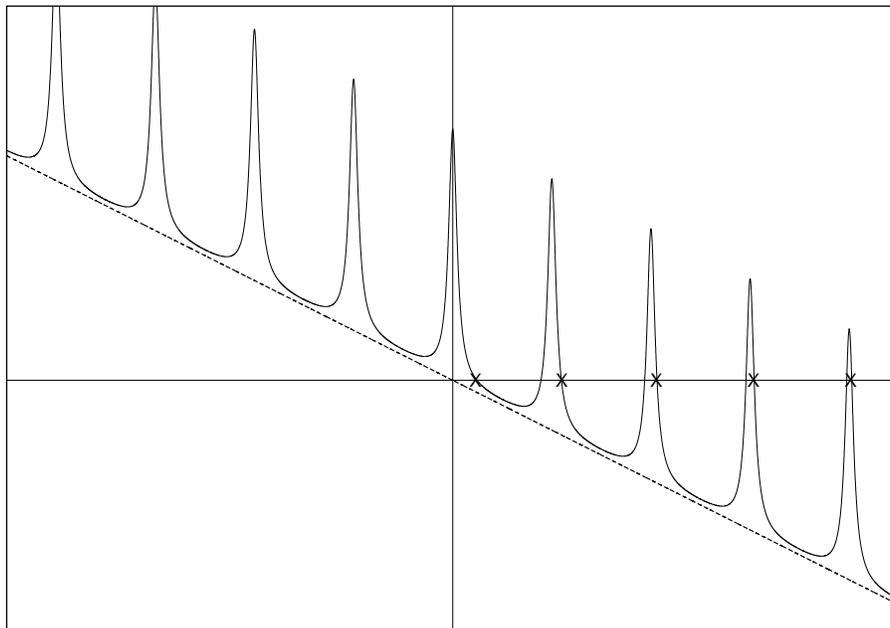
FIG. 2. Dependence of the ponderomotive force on the distance between the mirrors
